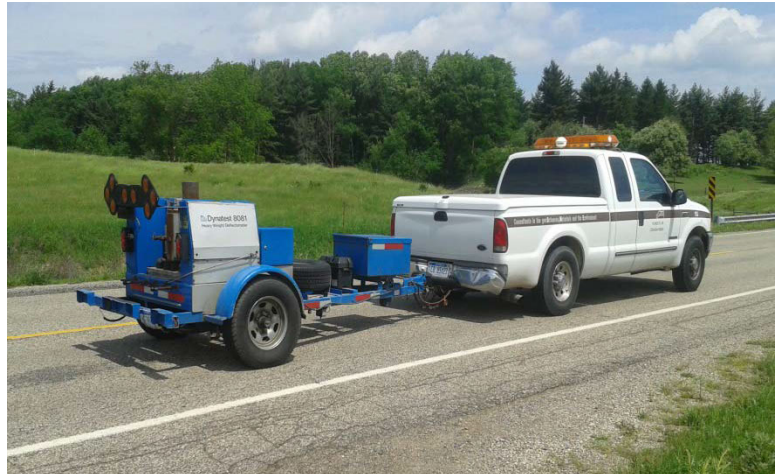
Falling Weight Deflectometer (FWD) testing performed by Soils & Materials Engineers, Inc. on Marshall Road, Walton Township
